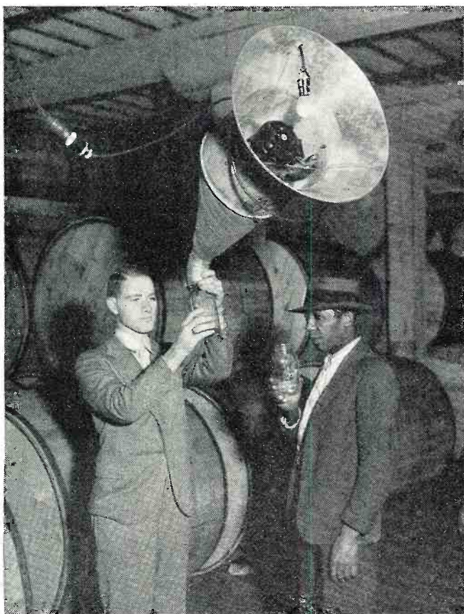
An electronically controlled trap, with light as bait, reduces the number of tobacco destroying insects in a warehouse.
